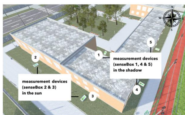
Figure 3. Experimental set-up (Screenshot of IVR) and temperature values recorded in the afternoon
