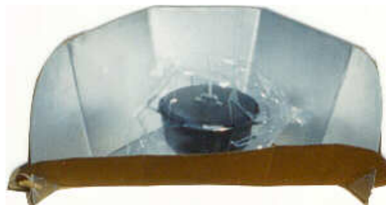
Figure 4. A solar cooker constructed from cardboard with a pot centred inside a plastic bag
